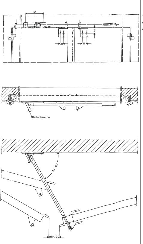
The closing sequencer has the task, to control the closing of 2-leaf fire doors in the right sequence.
